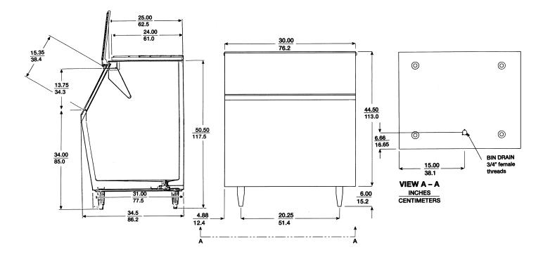
NOTE: Allow 6" minimum space at back for ice machine ventilation and utility connections.
